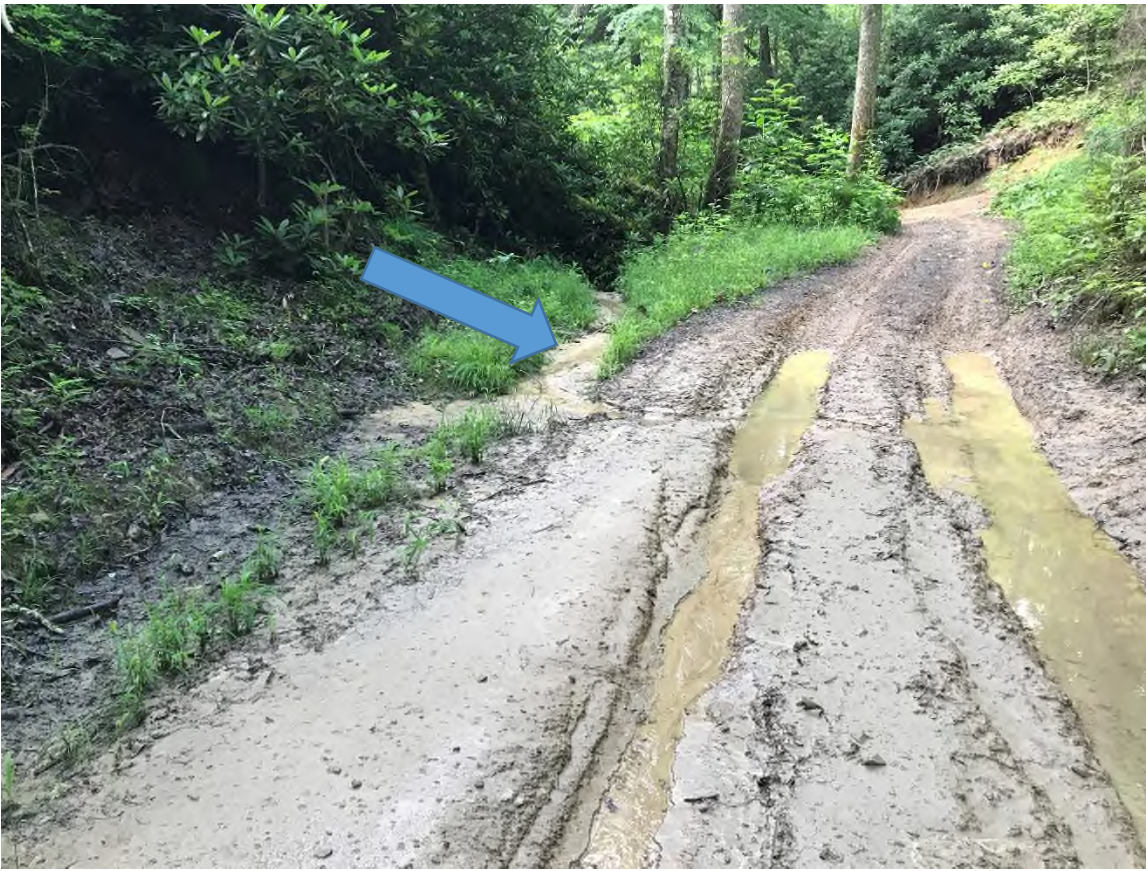
Figure 06 (Sediment deposition observed in unnamed tributary of Laurel Fork adjacent to Trail 16; 37.30075° , -81.38333° )
